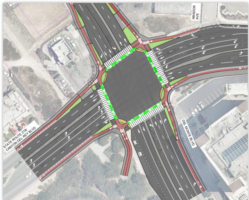
Figure 4.10 – Del Monte Blvd Protected Intersection
