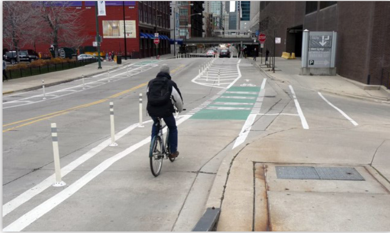
Figure 4.8 – Protected Cycletrack with Posts Example 3
