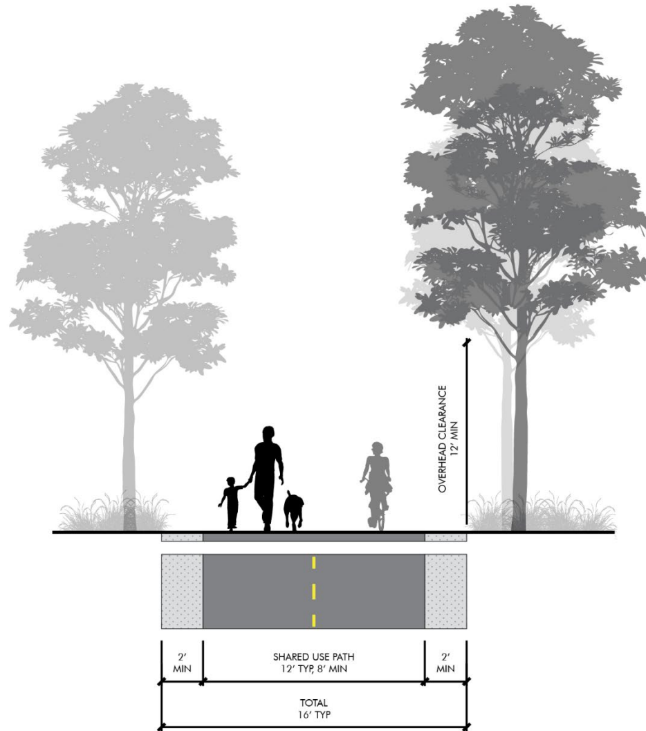
Figure 2-135 Example Cross-Section: FORTAG with No Side Path
