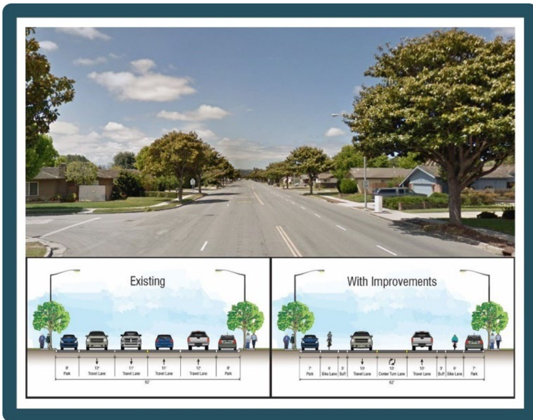
Figure 1: Roadway Configuration Before and After the improvements
